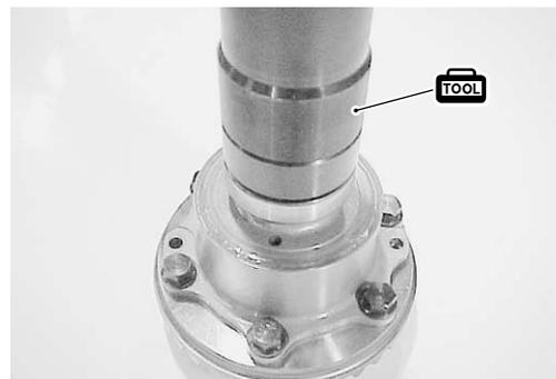
**FRONT DRIVE GEAR CASE OIL SEAL**
