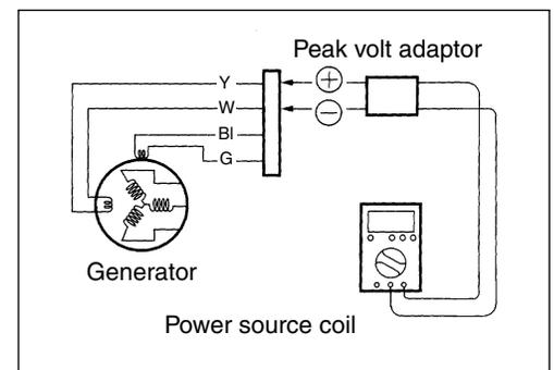
**PICKUP COIL AND POWER SOURCE COIL RESISTANCE**
