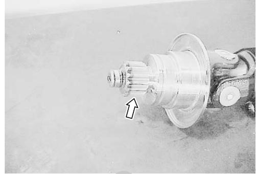
Inspect the universal joint and outer surface of the bearing for scuffing, wear and damage. If any defects are found, replace the bearings and universal joint as a set.
