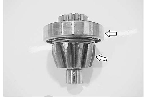
Check the gear case bearings for wear or damage.
