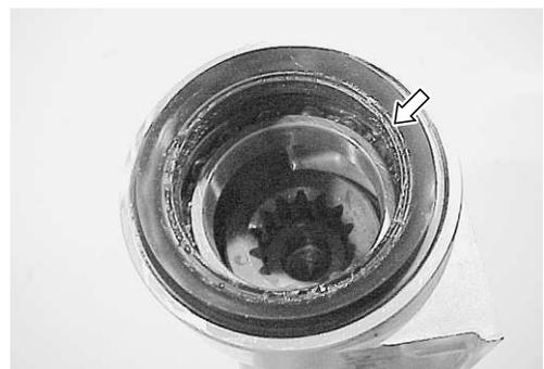
Check the outer race play and smooth rotation of the bearing by hand while it is on the pinion gear shaft.
