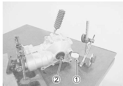
Remove the oil filler cap and measure the backlash of the differential ring gear using the horizontal type dial gauge ① and proper size of wooden piece or plastic piece ②, as shown. Take backlash readings at three places while turning the ring gear slightly in each direction and securely holding the pinion gear. Read the total backlash on the dial gauge.
