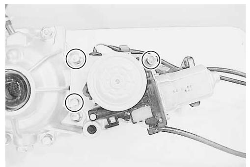
**2WD/4WD SHIFTING PINION AND SWITCH**
