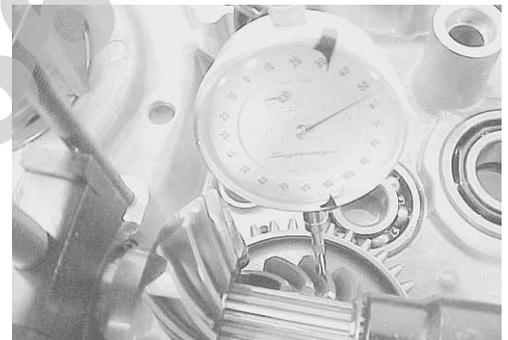
Measure the backlash by turning the drive bevel gear shaft in each direction, reading the total backlash on the dial gauge. If the backlash is not within specification, the shim must be changed and the backlash should be re-checked until correct. Refer to the chart at the right for appropriate shim thickness.
