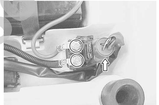
Apply 12 V to the terminals and check for continuity between the positive and negative terminals using the multi circuit tester. If the starter relay clicks and continuity is found, the relay is ok.
