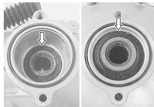
Check the gear case and case cover bearings for wear or damage.
