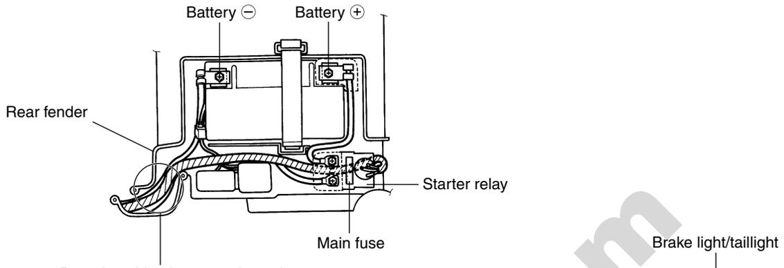
Pass the wiring harness above the ground wire and starter motor lead wire, and set them to the groove of the rear fender.
