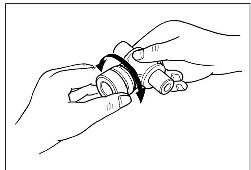
Inspect the front and rear output shafts for distortion. If distortion is found, replace the front or rear output shaft with a new one.
