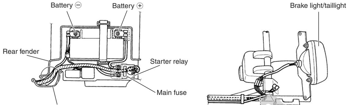
Pass the wiring harness above the ground wire and starter motor lead wire, and set them to the groove of the rear fender.
