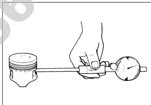
Using a micrometer, measure the piston pin outside diameter at three positions.
