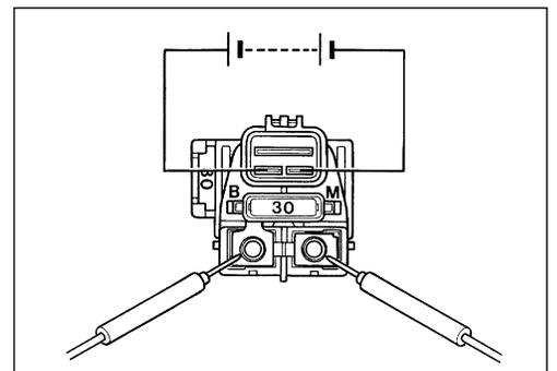
Measure the relay coil resistance between the terminals using the multi circuit tester. If the resistance is not within the specified value, replace the starter relay with a new one.
