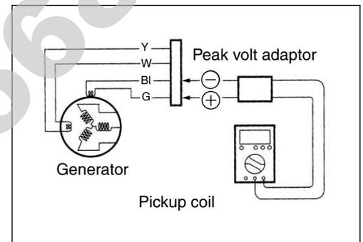
If the peak voltage on the generator coupler is within the specification, but on the CDI unit coupler is not within specification, replace the wire harness with a new one. If both peak voltages are out of specification, replace the generator with a new one.
