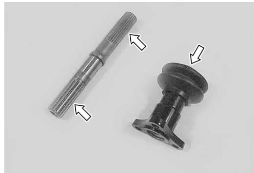
Inspect the parking cam, thrust bearing and return spring for any flaws or damage. If any defects are found, replace the cam, bearing and spring with the new ones.
