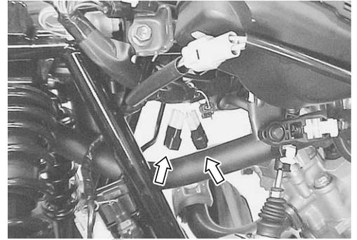
Measure the voltage between the terminals using the multi circuit tester as indicated in the table below.
