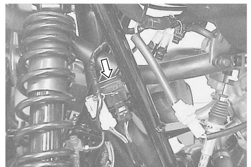
First check the insulation between ② and ③ and between ① and ③ terminals with the tester.
