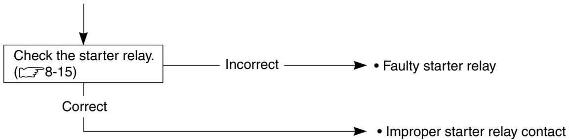
The starter motor runs when the transfer gear position is in neutral, but does not run when the transfer gear position is in any position other than neutral, with the parking brake lever grasp firmly.
