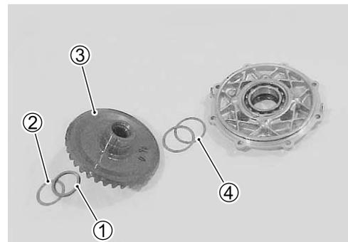
**GEAR CASE COVER/GEAR CASE [FINAL ASSEMBLY]**
