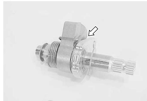
Inspect the oil seal for wear or damage. Check the inner race play and smooth rotation of the bearing by hand while it is in the case. If any defects are found, replace the oil seal and bearing with the new ones.
