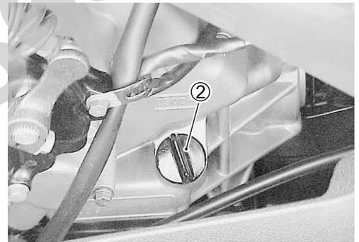
**U** Engine oil drain plug: 23 N·m (2.3 kgf·m, 16.5 lb·ft)
