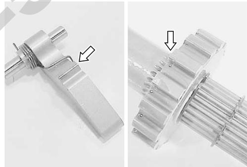
Inspect the splines of rear drive shaft and its coupling joints for wear or damage.
